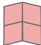
This is a famous fold called the Miura-ori. Its stiff elements are the panels, and its flexible elements are the sides/folds. Note that the panels are parallelograms.
