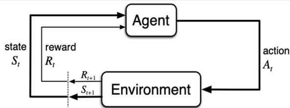
Figure 1. This chart shows the agent-environment loop. The agent, the learner, in this case is the lunar lander and behavior characteristics (BCs) change based on the agent's interactions with the environment. As the agent does the action the environment changes then it tells the agent its new state and it gets a reward, then this loop continues until the agent maximizes its reward.
