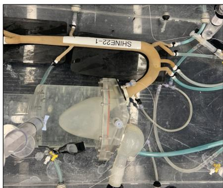
Figure 1: Artificial aorta, left ventricle (LV) and left atrium (LA) in the mechanical setup. PC: Christopher Lopez
