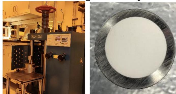
Fig. 3 (right): Perovskite oxide mounted on stage. Fig. 4 (left): cold isostatic pressing (CIP) unit for shaping targets. PC: Mythili Surendran
