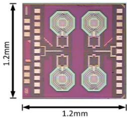
Fig. 1. Magnetic particle spectrometer IC with on-chip inductors.
