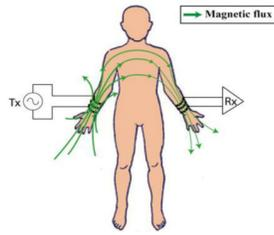
Fig. 2. Magnetic coupling data transfer link in a WBAN
