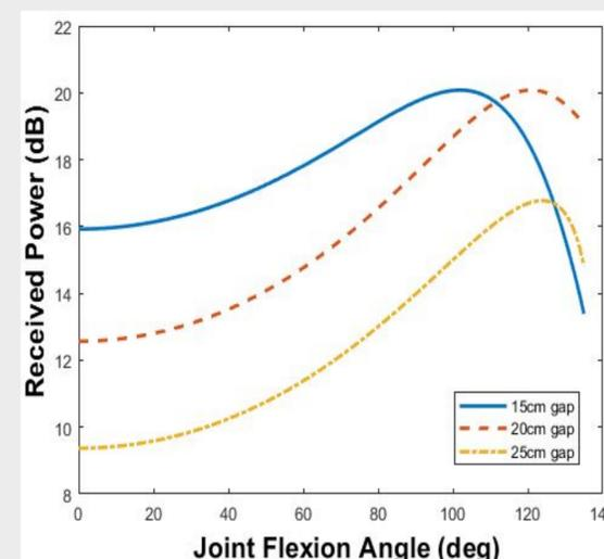
**Fig. 4. Received power (dB) as function of joint flexion angle (degrees) for three different joint to transmitter gap separation.**
