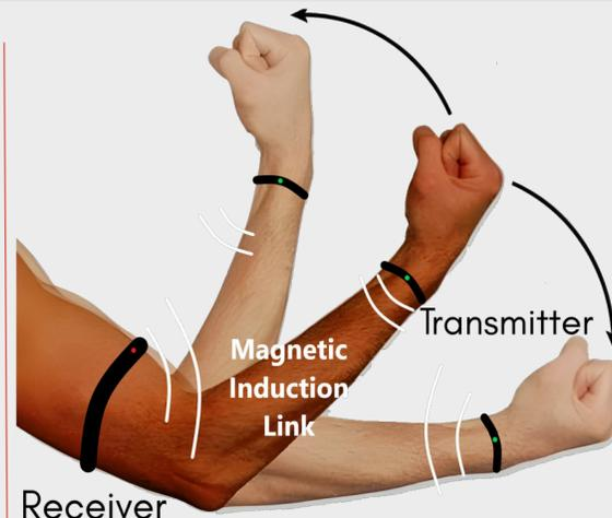
**Fig. 1. Joint flexion monitoring using wearable magnetic coils.**
