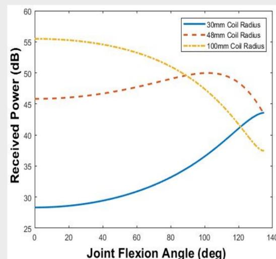
**Fig. 3. Received power (dB) as function of joint flexion angle (degrees) for three different TX/RX coil radii.**
