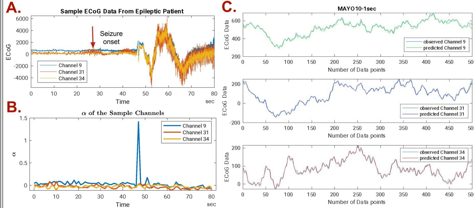
**Figure 2 System Identification.** Fig. 2A Shows sample data from MAYO10 patient exhibits seizure onset at 20 sec. Fig. 2B The order of the systems are fractional orders, and they demonstrates significant difference from 0. Fig. 2C One-step prediction for ECoG data for one second shows that the fractional order system can accurately predict data. \*PC: Julia G.
