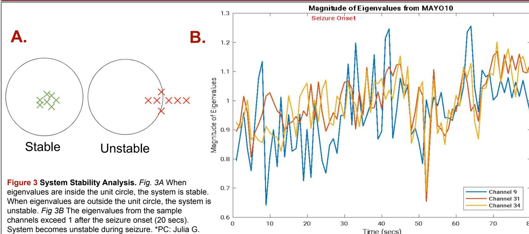
**Figure 3 System Stability Analysis.** Fig. 3A When eigenvalues are inside the unit circle, the system is stable. When eigenvalues are outside the unit circle, the system is unstable. Fig. 3B The eigenvalues from the sample channels exceed 1 after the seizure onset (20 secs). System becomes unstable during seizure. \*PC: Julia G.
