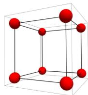
Figure 2. Model of Simple Cubic
