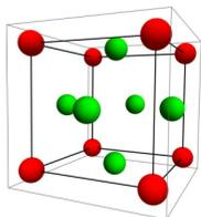
Figure 3. Model of Face Centered Cubic
