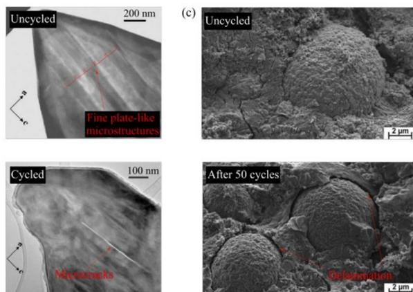
Figure 1. Intercalation material before and after being cycled
