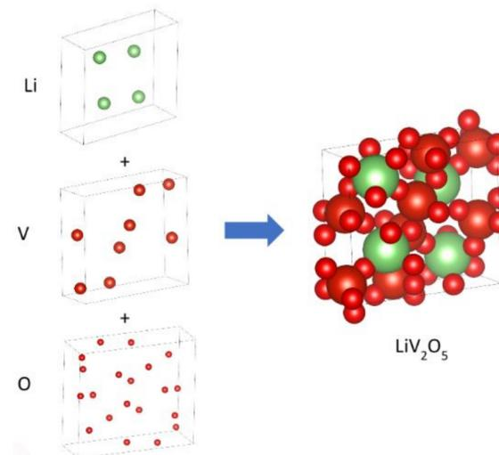
Figure 5. Visual representation of  $\text{LiV}_2\text{O}_5$
