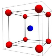
Figure 4. Model of Body Centered Cubic
