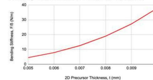
Figure 9. Bending stiffness plotted against various 2D precursor thicknesses
