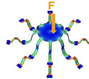
Figure 6. 3D structure deforming under load. The deformation under load is a function of the structure and material properties.
