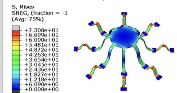
Figure 3. FEA of stress distribution of a 3D structure formed by mechanical buckling. Different colors correspond to different levels of stress generated in buckling process.
