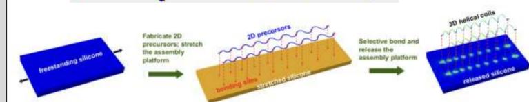
Figure 2. Schematic illustration of the mechanical buckling process to form 3D structures Reference: Science, 347.6218 (2015): 154-159.
