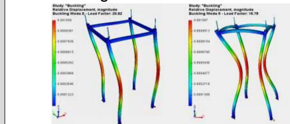
Figure 1. A structure under a load exhibiting the characteristic deformation of buckling
