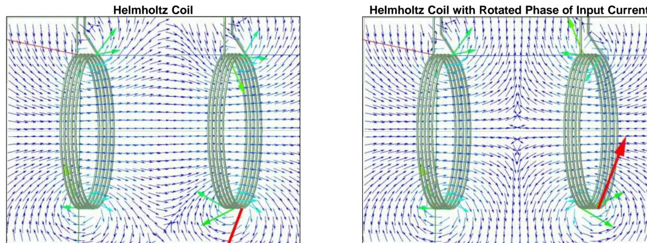
Constant field passing through the two currents. Each coils has 5 turns, and the distance between each coil is 0.5cm. Arrows in graph represent magnetic field vector.
