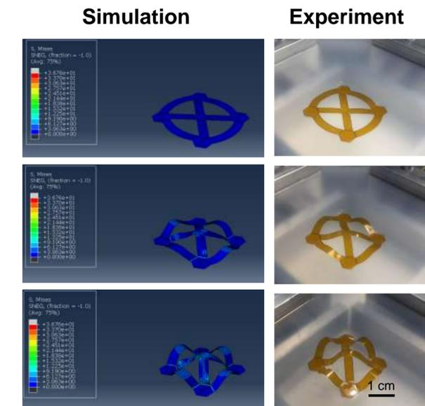
Figure 4. Abaqus simulation compared to real life images of a 3D structure formed by compressive buckling based on design in Figure 3, Amado Ochoa
