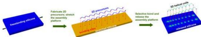
Figure 1. Schematic illustration of the mechanical buckling process to form 3D structures. Reference: *Science*, 347.6218 (2015): 154-159.
