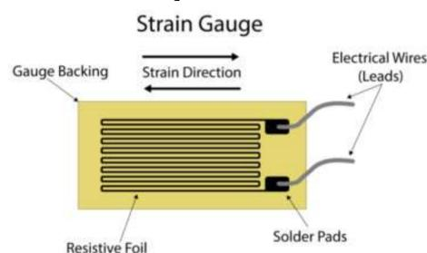
Figure 2. Piezoresistive Sensor, sensor attached to mesostructure able to read forces applied by displaying as change in electric current, Michigan Scientific Corporation
