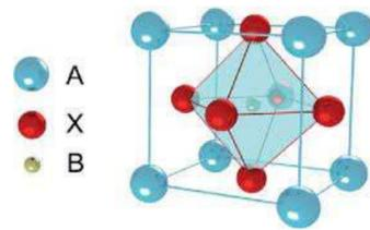
Figure 1. Perovskite crystal structure
