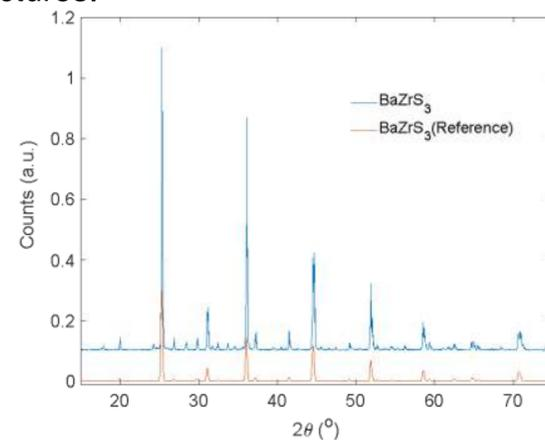
Figure 4. X-ray diffraction of BaZrS<sub>3</sub> and reference data.
