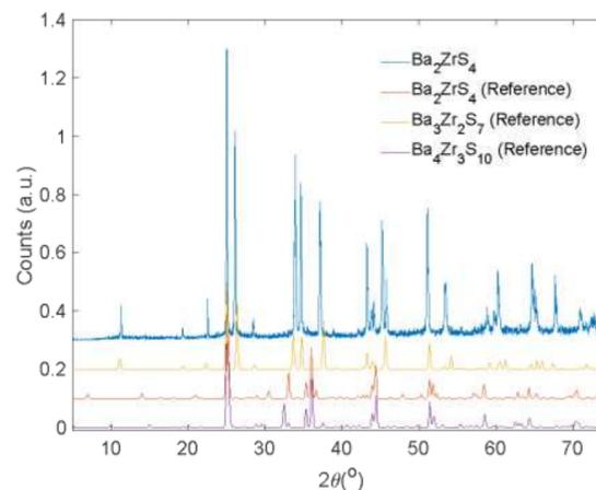
Figure 5. X-ray diffraction of Ba<sub>2</sub>ZrS<sub>4</sub> and reference data.
