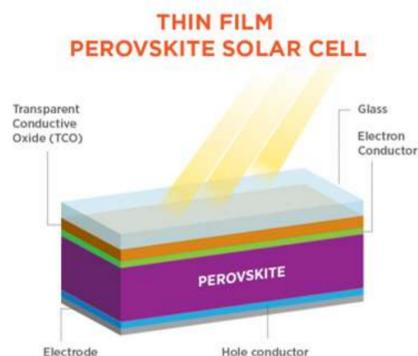
Figure 3. Model of a perovskite solar cell
