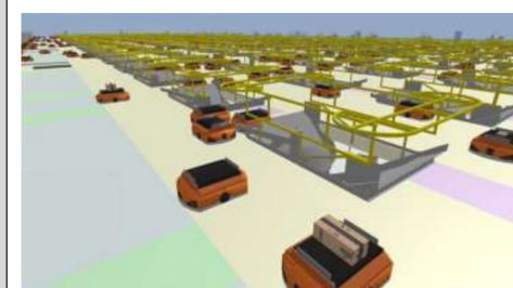
**Fig. 1:** Simulation of coordination between robots at an Amazon warehouse
