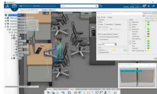
In figure 3, we created a manikin on a construction site behind the robot. The manikin is also carrying a control unit weighing about 3 kg.
