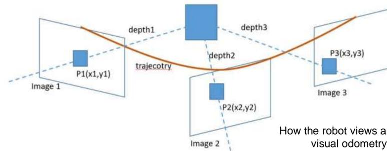
How the robot views and uses visual odometry
