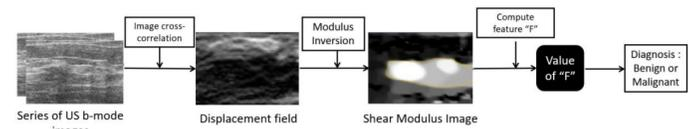
Standard Ultrasound based Elastography workflow
