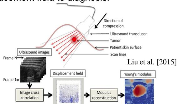
Figure 1 : Elastography process
