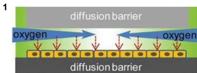
Model of microfabricated device designed to replicate hypoxia (lack of oxygen) in tumors. Yellow rectangles represent MCF-7 breast cancer cells. Cells near the edge of the device receive more oxygen than cells near the center.
