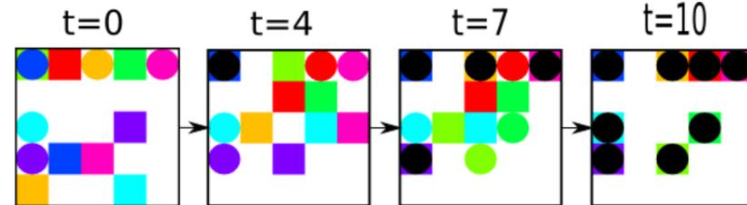
This example is our second step of multi agent path finding with many agents in a confined space. The colored squares indicate the robots and the corresponding circle is the goal it must reach. T indicates the time step.
