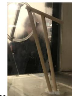
Figure 6: Our model of the structure in the Dryden Wind Tunnel. We tested the apparatus by itself to measure its drag. PC: Saakar Byahut.
