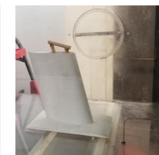
Figure 7: Shroud over apparatus. Our proposed solution was an aerodynamic shroud that would encompass the two cylinders to reduce their drag. We tested the drag of the apparatus with the shroud on top. PC: Saakar Byahut.
