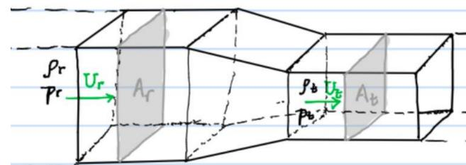
Figure 5: Wind Tunnel. This is a model of a general wind tunnel. The smaller section (called the test section) is the area in which we tested our set-up. PC: Saakar Byahut.
