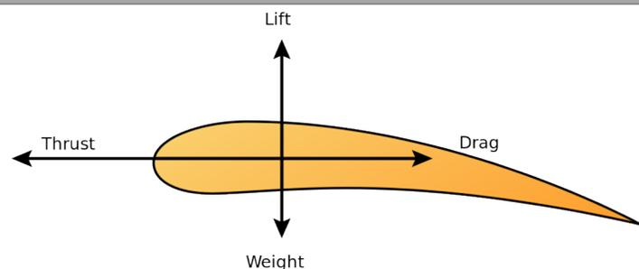
Figure 1: Aerodynamic Forces. These four forces act on all aircraft. <[https://en.wikipedia.org/wiki/Aerodynamic\\_force](https://en.wikipedia.org/wiki/Aerodynamic_force)>
