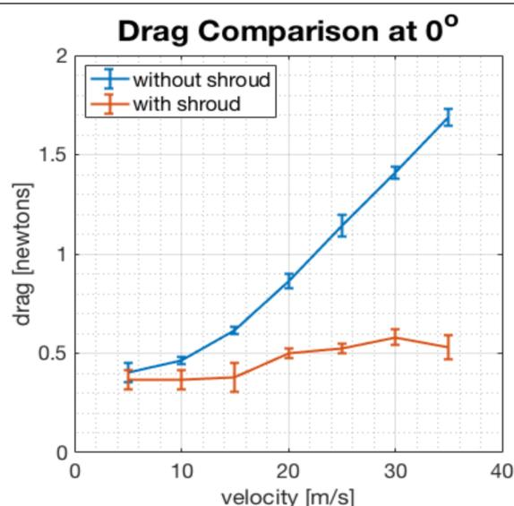
Figure 4: Results of Testing. It can be concluded that our shroud definitively reduced the drag of the apparatus. PC: Manaeha Rao.
