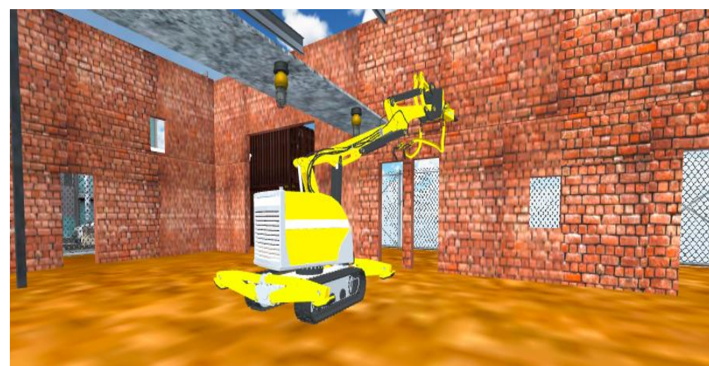
Computer animated destruction robot, Brokk, within the construction site PC: Erica De Guzman
