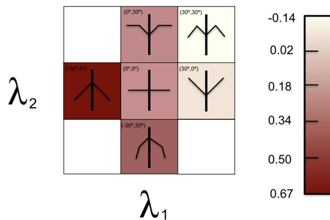
The diagram above depicts the six various wing configurations positioned by their respective inboard and outboard angles. The color gradient illustrates the static margin value for each glider wing. The graph below shows the average  $L/D$  for two different speeds tested on the wings.
