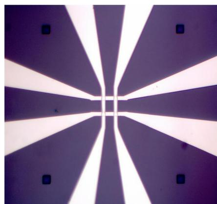
Figure 7: This is a picture of a 2x2 memristor crossbar taken under a microscope. Notice the 4 intersection points in the center: each crossbar is joined to a large metal electrode where a probe can be placed to apply a voltage across the crossbar. PC: Brian Chu
