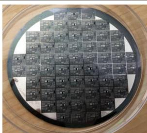
Figure 1: A dense lab-made sample of computer chips PC: Brian Chu
