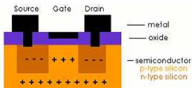
Figure 3: The structure of a traditional silicon transistor <<https://bit.ly/2LudfWk>>
