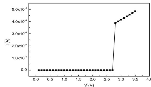
Figure 8: An IV curve plotting voltage inputs against current outputs for the memristor; to calculate the resistance, we take the reciprocal of the slope, or  $V/I$ . The flat line from 0-2.75V represents a state of high resistance; once the voltage reaches the threshold of 2.75V, the memristor switches to a low resistance state and turns on. PC: Hefei Liu
