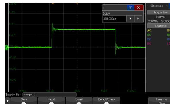
Figure 9: A pulse that I generated using a Quartus II FPGA program that can control the memristor's state by applying/stopping the voltage input at specific intervals. The program is crucial as it prevents the memristor voltage from becoming too strong and causing the device to stop functioning. PC: Brian Chu
