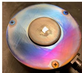
Figure 2a. VO<sub>2</sub> thin film on STO substrate. (PC: Oscar Chou)
