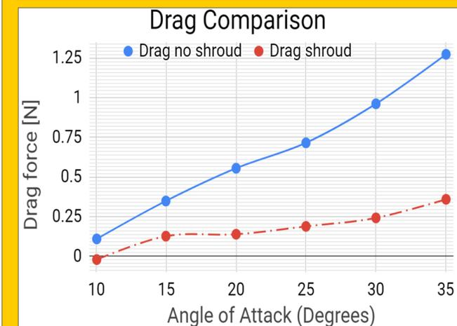
Evidently, the drag of the shrouded apparatus was significantly lower than the bare apparatus. The drag force was reduced by 70% when tested at speeds of 35 m/s.
