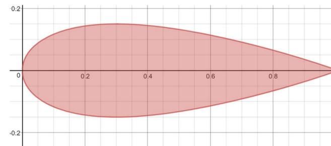
NACA 0030 airfoil, 0.3 units thick and 1 unit chord length
