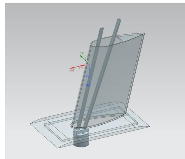
CAD design of the shroud and the setup
