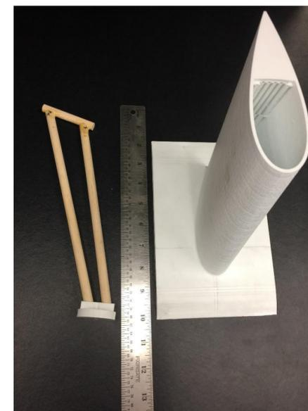
3D printed shroud and model of the setup, chord length:  $c = 5.25$  in., height:  $b = 7.19$  in.
