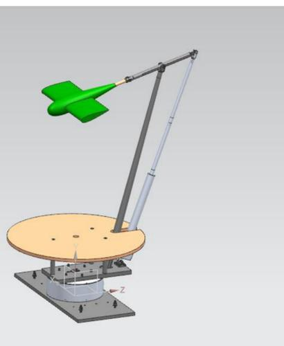
CAD design of the setup in the Dryden Wind Tunnel.
