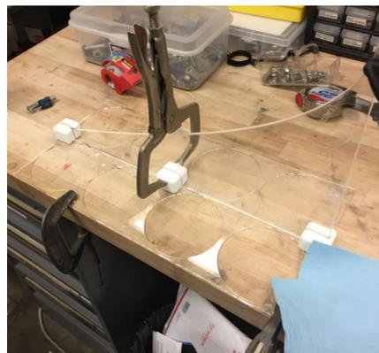
The parabolic support being glued to the acrylic sheet. The alignment blocks are the small white squares. PC: Brody Bishop
