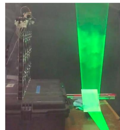
Using PIV to visualize a shear pattern, with the top rows of fans blowing harder than the bottom rows. PC: Sarah Fry
